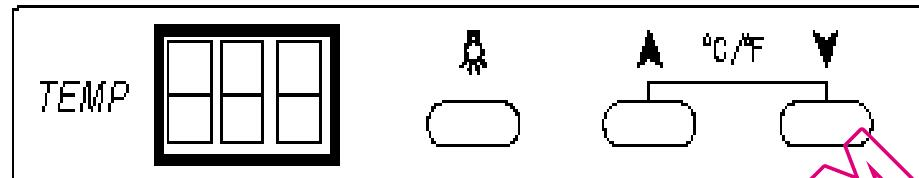
When the power is connected, the cooling system starts to work. The temperature is adjusted in the range of 4°C—18°C in the cabinet.
